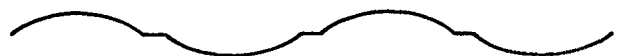
Fig. 28B - Smaller Amplitude Sine Wave with same amount (higher %) of Crossover (notch) Distortion.
